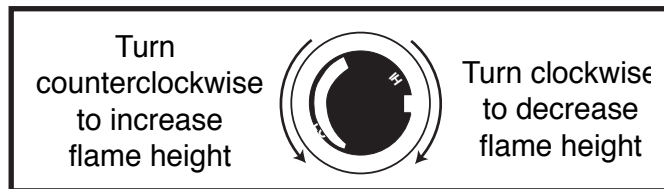
Fig. 42 Flame adjustment knob for SIT valve.
